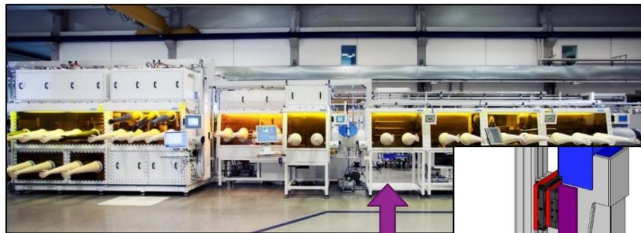
HSI next to ALD chamber in  $15 \times 15 \text{ cm}^2$  printed electronics processing
